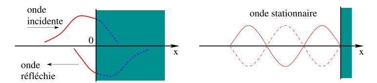
Let the incident plane wave be  $F_i(t-x/c)$ , the reflected wave  $G_r(t+x/c)$  is also plane. The total wave is  $u(t,\mathbf{r})=F_i(t-x/c)+G_r(t+x/c)$ .
