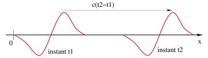
**Example**: The vibration  $F(t) = \cos(\omega t)$  yields  $u(t,x) = \cos(\omega t - kx)$   $\omega = 2\pi f$  is the angular frequency; f is the frequency (in Hz).  $k = \omega/c = 2\pi/\lambda$  is the wavenumber;  $\lambda$  is the wavelength.
