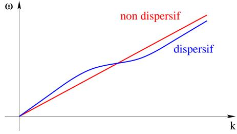
For a wave packet:  $u(t,x) = \frac{1}{2\pi} \int_{-\infty}^{\infty} \tilde{F}(\omega) \exp(\mathrm{i}(\omega t - k(\omega)x)) d\omega$
