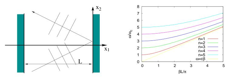
In order for the superposition of two harmonic plane waves to satisfy boundary conditions on the mirrors, phase matching must be observed:
