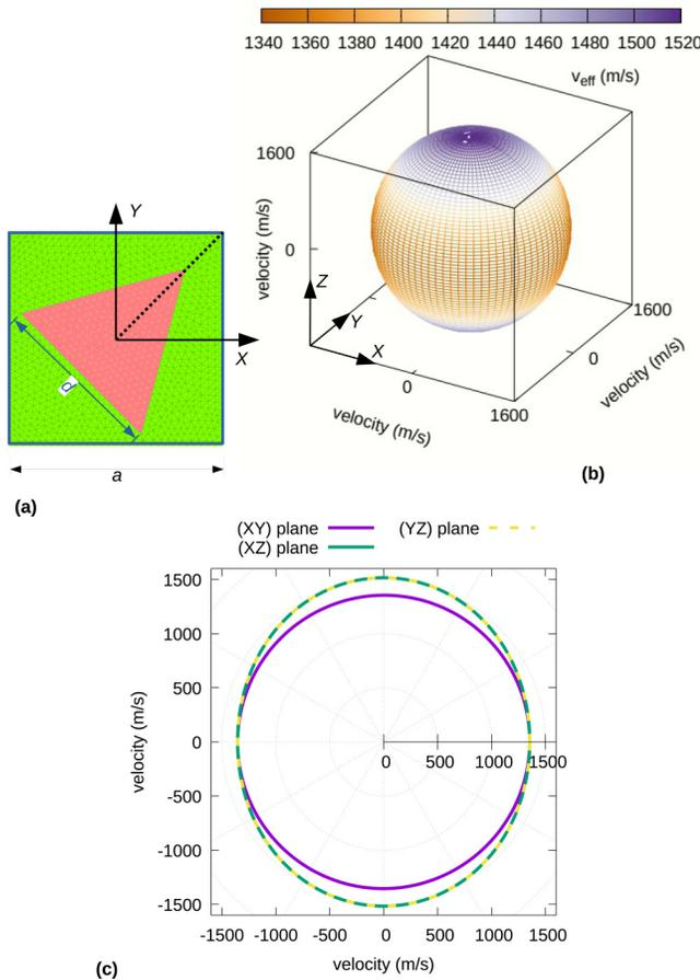
**FIG. 2.** A 2D square-lattice sonic crystal composed of triangular steel rods in water. (a) The triangular rods are rotated by  $45^\circ$  with respect to the  $X$  axis. The ratio of the length of the equilateral triangle to the lattice constant is  $d/a = 0.8$ . The crystal is orthotropic. (b) Effective velocity surface. (c) Cross sections through the symmetry planes of the crystal.
