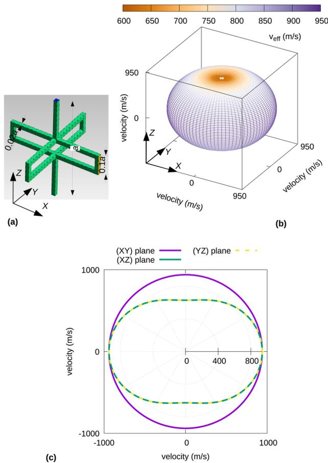
**FIG. 6.** (a) A 3D sonic crystal composed of a periodic array of waveguides containing water. The crystal is orthotropic with two independent tensor elements. (b) Effective velocity surface. (c) Cross sections through the symmetry planes of the crystal.
