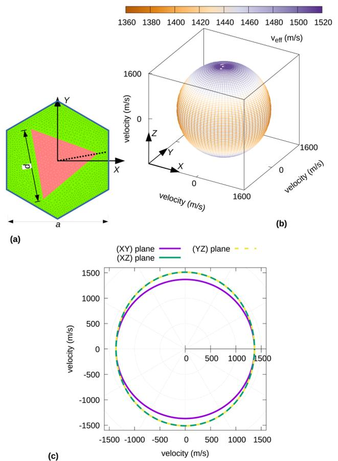
**FIG. 3.** (a) A 2D hexagonal-lattice sonic crystal composed of triangular steel rods in water. The triangular rods are rotated by  $10^\circ$  with respect to the  $X$  axis. The ratio of the length of the equilateral triangle to the lattice constant is  $d/a = 0.7$ . The crystal has a  $C_3$  symmetry and is transverse isotropic. (b) Effective velocity surface. (c) Cross sections through the symmetry planes of the crystal.
