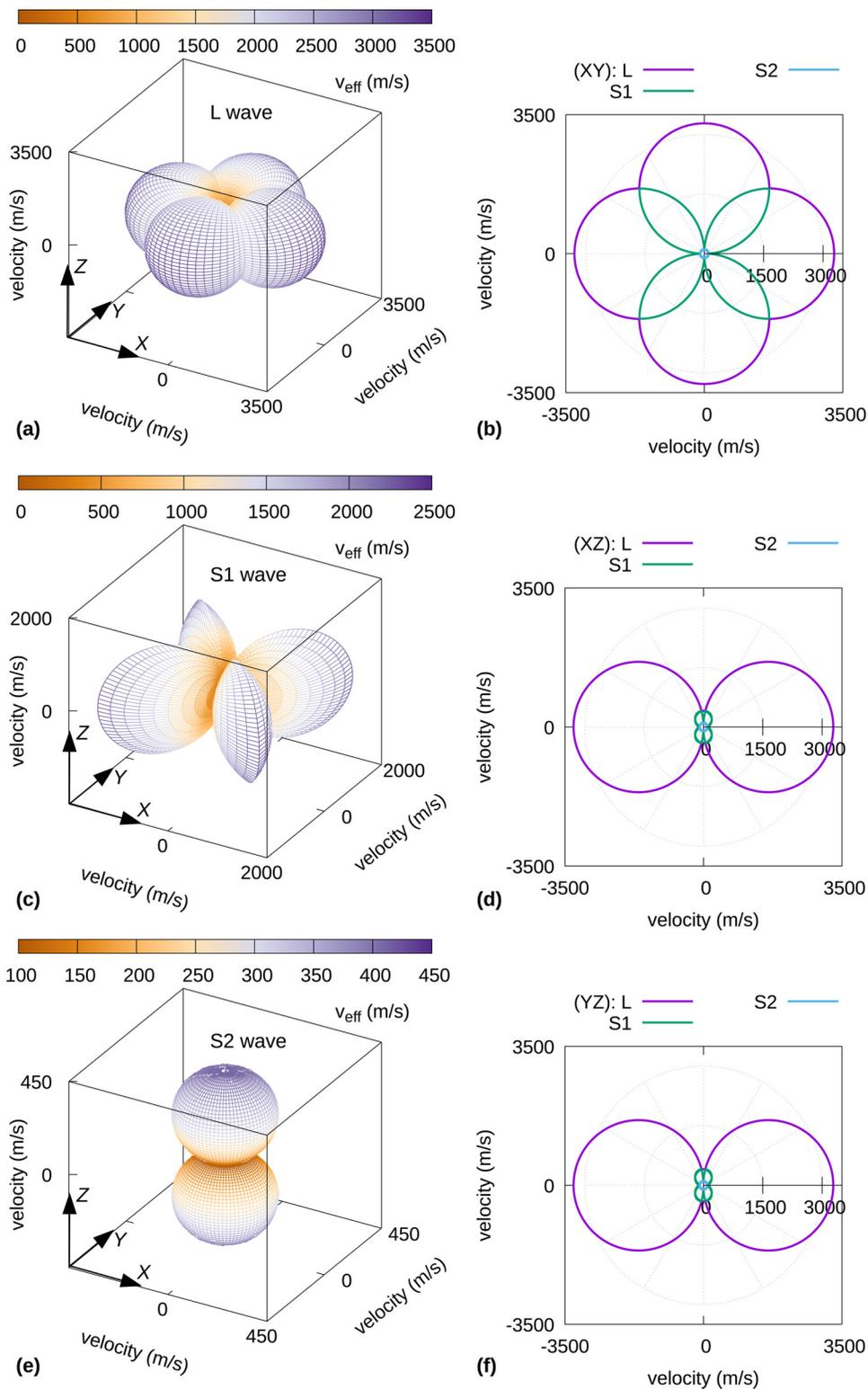
**FIG. 10.** A 3D phononic crystal composed of a periodic array of steel bars, with the same mesh as in Fig. 6. The crystal is orthotropic with three symmetry planes. (a),(c),(e) Effective velocity surfaces for the three elastic waves. (b),(d),(f) Cross sections through the symmetry planes of the crystal.
