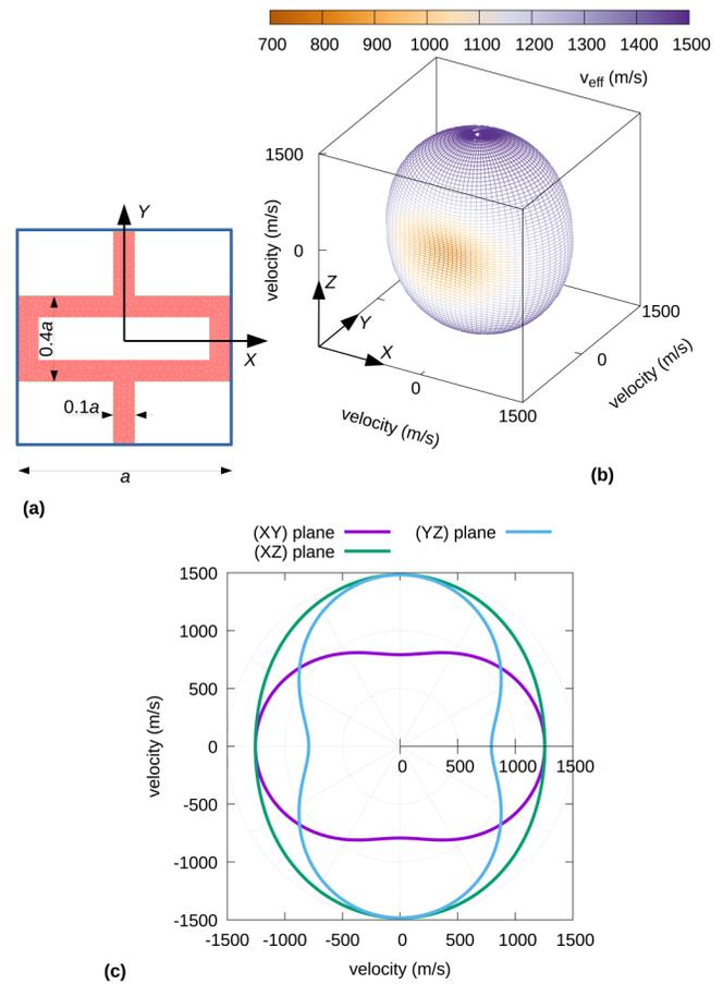
**FIG. 5.** (a) A 2D sonic crystal composed of a periodic array of waveguides containing water. The crystal is orthotropic with three independent tensor elements. (b) Effective velocity surface. (c) Cross sections through the symmetry planes of the crystal.
