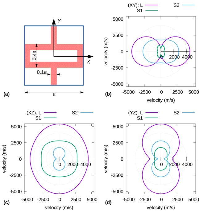
**FIG. 8.** (a) A 2D phononic crystal composed of a periodic array of steel bars. The crystal is orthotropic. (b)–(d) Cross sections of the three effective velocity surfaces through the symmetry planes of the crystal. In-plane (XY), the longitudinal velocity becomes smaller than the S2 shear velocity in a certain angular range.
