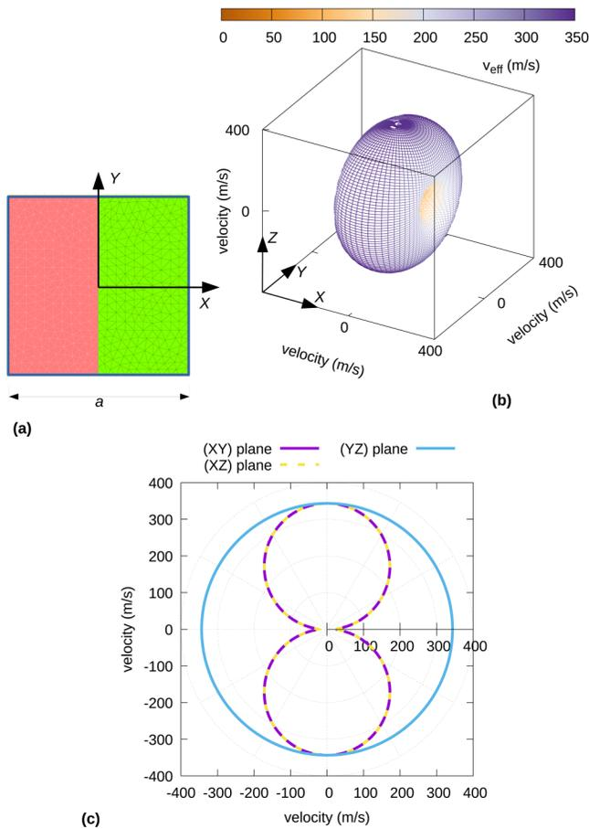
**FIG. 4.** (a) A laminar 1D sonic crystal composed of alternated layers of water and air with equal thickness. The structure is invariant along axes  $Y$  and  $Z$ . The crystal is orthotropic with two independent tensor elements. (b) Effective velocity surface. (c) Cross sections through the symmetry planes of the crystal.
