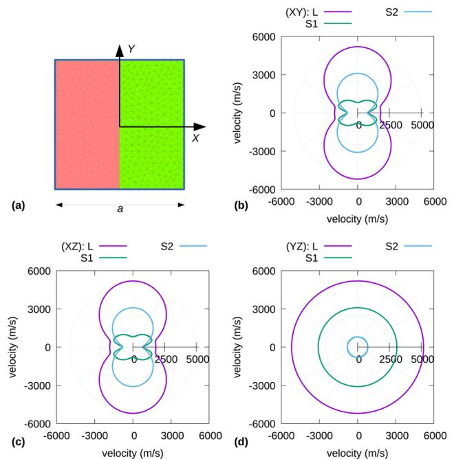
FIG. 7. (a) A laminar 1D phononic crystal composed of alternated layers of steel and epoxy with equal thickness. The structure is invariant along axes  $Y$  and  $Z$ . The crystal is orthotropic. (b)–(d) Cross sections of the three effective velocity surfaces through the symmetry planes of the crystal.
