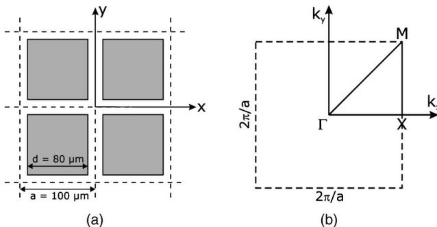
FIG. 1. (a) Cross section of a biperiodic solid-solid phononic band-gap material, consisting of quartz rods in epoxy. (b) First Brillouin zone in the  $(k_x, k_y)$  plane.
