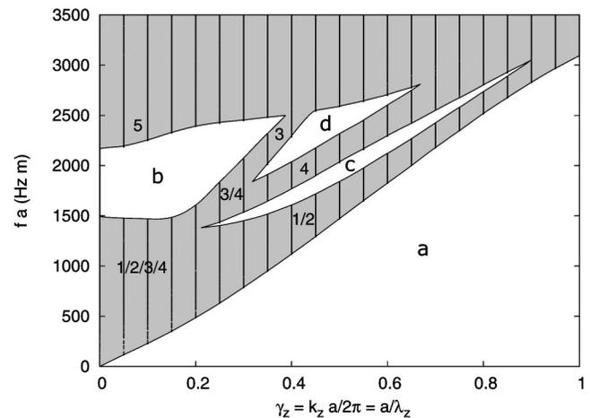
FIG. 2. Projection of the phononic band structures in the  $(k_x, k_y)$  plane onto the  $(k_z, f)$  plane. Numbers indicate the positions of particular branches labeled in Fig. 3. Delimited white regions indicate absolute stop bands in the  $(k_x, k_y)$  plane.
