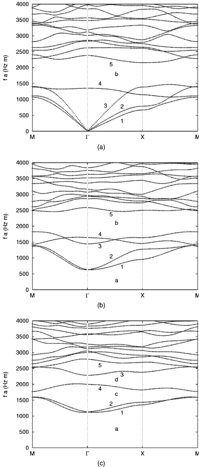
FIG. 3. Dispersion curves along the  $M$ - $\Gamma$ - $X$ - $M$  path shown in Fig. 1(b), for (a)  $\gamma_z=0$ , (b)  $\gamma_z=0.25$ , and (c)  $\gamma_z=0.4$ . The first five branches are numbered in the order of their appearance in the  $\gamma_z=0$  dispersion diagram.
