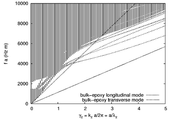
FIG. 4. Same as Fig. 2 but for an enlarged range of  $k_z$  values. Bulk-epoxy longitudinal and transverse modes are indicated.
