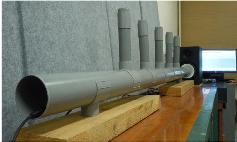
**Figure 1.** Photograph of one of the 1D phononic crystal samples. The 2 m long tube has a diameter of 10 cm.
