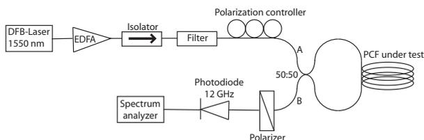
Fig. 1. Experimental setup for observing guided acoustic wave Brillouin scattering.
