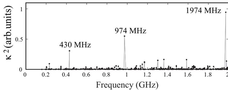
Fig. 4. Elasto-optic coefficient as a function of the acoustic frequency for the perfect microstructure.
