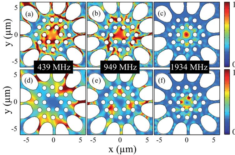
Fig. 3. Numerical calculation (color plot) of the strain energy density distribution (a-c) and the kinetic energy density (d-f) of the 439, 949 and 1934 MHz acoustic modes.
