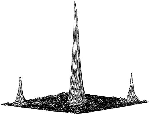
Fig. 3. Correlation function obtained with the proposed nonlinear filtering (nonlinear JTC) technique.
