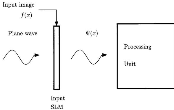
Fig. 1. Coding scheme of an input image with an EASLM.  $f(x)$  denotes the input signal sent to the EASLM, and  $\Psi(x)$  is the optical field after passage through the EASLM.
