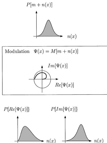
Fig. 2. Modification of the probability density of an input noise  $n(x)$  when the modulation law is of the form  $M(z) = z \exp(iKz)$ .  $m$  is the signal without noise and  $\text{Re}(\cdot)$  [ $\text{Im}(\cdot)$ ] indicates the real part (imaginary part) of a complex number.
