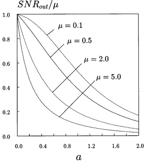
Fig. 6. Ratio of output signal-to-noise ratio to input signal-to-noise ratio as a function of  $a$  for different values of  $\mu$ .
