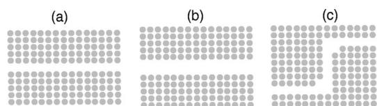
FIG. 1. Cross sections of waveguides formed by removing rods from an ultrasonic crystal made of steel rods immersed in water. (a) A one-period-wide straight waveguide (W1). (b) A two-period-wide straight waveguide (W2). (c) A one-period-wide bended waveguide.
