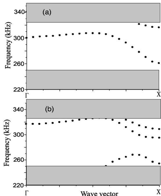
FIG. 4. Super-cell calculation of the dispersion relation for (a) waveguide W1 and (b) waveguide W2.
