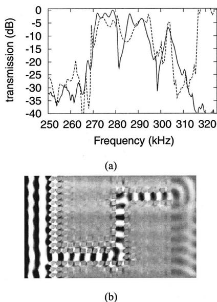
FIG. 5. (a) Same as Fig. 2(a) but for the one-period-wide bended waveguide of Fig. 1(c). (b) Calculated acoustic pressure averaged over one period at the frequency  $f=275$  kHz.
