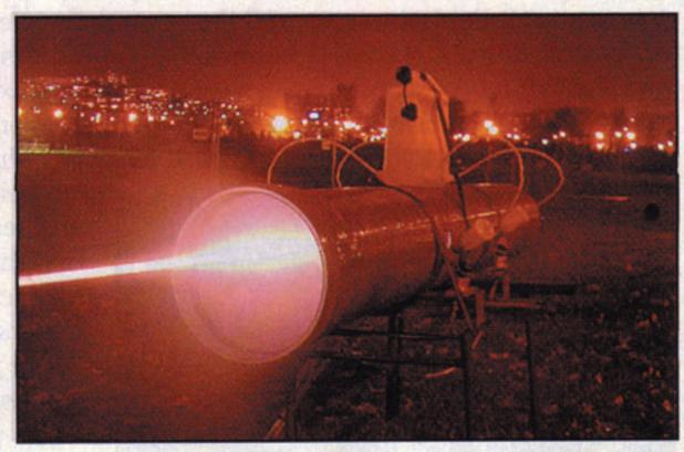
droplets of water or ink. Moreover, the filaments passed unscathed through a 0.35-m-long cloud chamber with an optical thickness as high as 3.2, corresponding to that of a cumulus or stratocumulus cloud, they reported.
