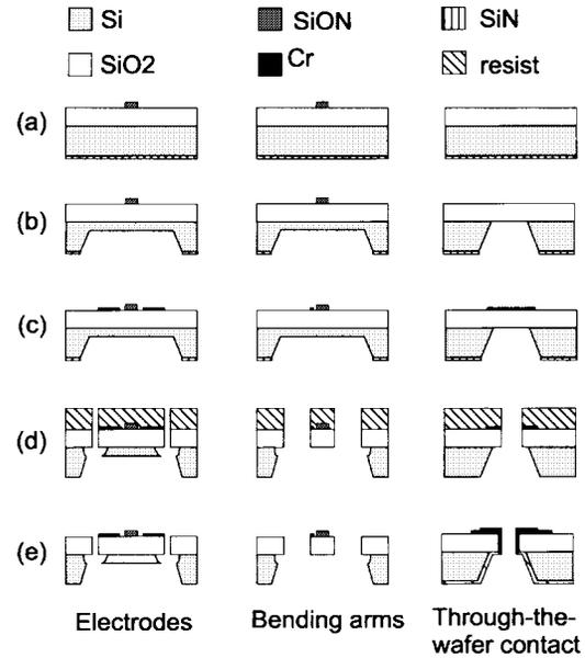
Fig. 8. Process for the upper wafer. The columns show the process along different cut of the wafer: (left) the electrode support, (middle) the bending arm, (right) the hole through the wafer that brings the electrode contact to the back of the wafer.
