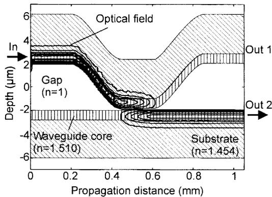
Fig. 3. BPM simulation showing the intensity of light along the waveguides in Fig. 2(b) with  $\lambda = 0.6 \mu\text{m}$ .
