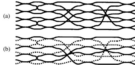
Fig. 1. Top-view of an  $8 \times 8$  optical switch matrix with (a) a conventional planar structure and (b) a two-level structure (full line and dotted line represents the waveguides on the upper and lower level, respectively).
