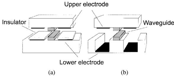
Fig. 6. (a) ON/OFF snapping actuator with insulated electrodes and (b) proportional actuator with recessed electrodes.
