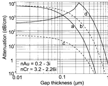
Fig. 5. Attenuation in a SiON rib waveguide coupled with an absorbing material through a low-index substance at  $\lambda = 0.633 \mu\text{m}$ . Attenuation for (a) the TE mode with chromium and air in the gap, (b) the TE mode with chromium and water ( $n = 1.31$ ) in the gap, (c) the TE mode with gold and water in the gap and, (d) the TM mode with gold and water in the gap.
