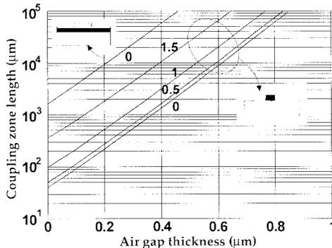
Fig. 4. Coupling length versus the air gap thickness and the misalignment for two types of waveguide at  $\lambda = 0.6 \mu\text{m}$  (the label of the curves gives the lateral misalignment between the two waveguides in  $\mu\text{m}$ ).
