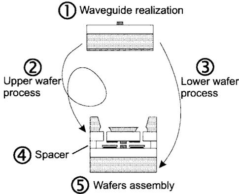
Fig. 7. Two wafers process for optical coupler on silicon.
