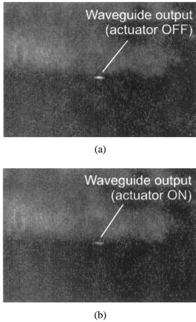
Fig. 12. Attenuator output in (up) OFF and (down) ON states for TE polarization.
