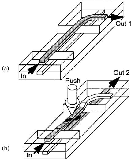
Fig. 2. Operation of the space driven evanescent coupler in (a) the through state and (b) the crossover state.
