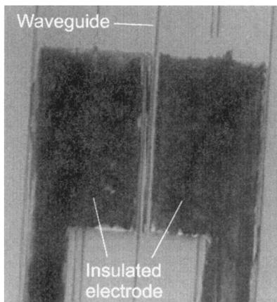
Fig. 10. Microphotograph of the lower wafer with the waveguide running between the insulated electrodes.
