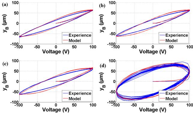
Fig. 6. Comparison between the displacement model of the end-effector tip B  $y_B$  given in (13) and experimental results for many sine voltages with an amplitude of 100V and with different frequencies where no force is applied: (a) 10Hz, (b) 50Hz, (c) 100Hz and (d) 500Hz.
