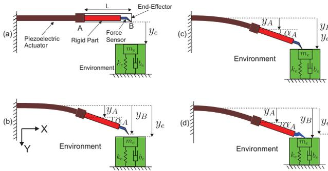
Fig. 1. Complete scheme of the smart finger and the environment: (a) without contact and without any applied voltage, (b) without contact and with an applied voltage, (c) just at contact ( $F_e = 0$ ) and with an applied voltage and (d) with contact ( $F_e \neq 0$ ) and with an applied voltage.
