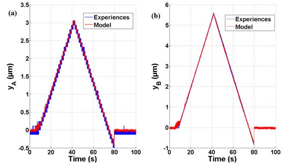
Fig. 7. Comparison between the displacement model at tips A and B,  $y_A$  and  $y_B$ , given in (13) and (3) and experimental results when a force is applied at the end-effector's tip B in static and with a short circuit on the electrodes of the actuator: (a) comparison at actuator's tip A,  $y_A$ , and (b) comparison at end-effector's tip B,  $y_B$
