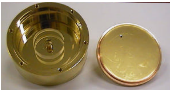
Fig. 2a : 26GHz-cavity before packaging
