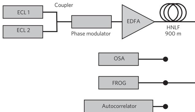
**Figure 3 | Experimental set-up.** ECL: external-cavity laser; OSA: optical spectrum analyser; FROG: frequency-resolved optical gating. HNLf: highly nonlinear fibre. EDFA: erbium-doped fibre amplifier.
