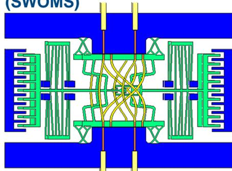
Legend: ■ Fixed parts ■ Moving parts ■ optic fiber
