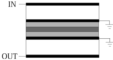
Fig. 4. Basic structure for a coupled resonator filter.
