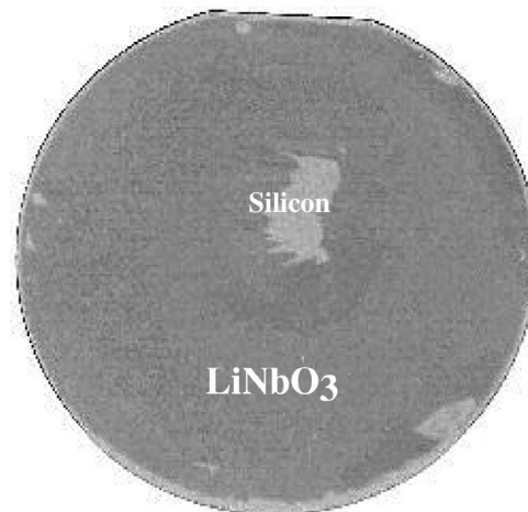
Fig. 7. Photo of a 4-in. wafer with almost perfectly transferred Y-cut LiNbO 3 top layer.
