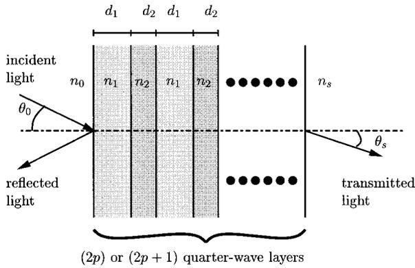
Fig. 1. Stack of alternate layers with refractive indices  $n_1$  and  $n_2$  and with respective thicknesses  $d_1$  and  $d_2$ .
