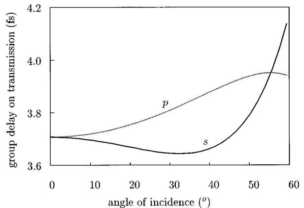
Fig. 4. Dependence of the asymptotic tunneling time on the angle of incidence for the quarter-wave stack of Fig. 3(a),  $\lambda_0 = 800$  nm, and  $q = 0$ .
