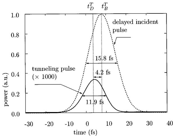
Fig. 6. Numerical simulation of the transmission of a 28-THz-bandwidth Gaussian pulse through barrier  $(HL)^{11}$  of Fig. 5 ( $20^\circ$  incidence,  $p$  polarization,  $\lambda_0 = 800$  nm, and  $q = 0$ ).
