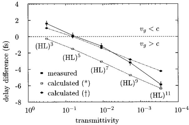
Fig. 5. Measured and calculated (\*) delay difference  $\Delta\tau$  ( $20^\circ$  incidence,  $p$  polarization,  $\lambda_0 = 800$  nm and  $q = 0$ ) in the experiment of Spielmann *et al.*<sup>4</sup> Calculated (†)  $\Delta\tau$  with the present theory.
