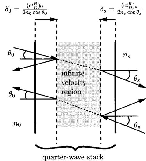
Fig. 2. Equivalent reflection planes describing the reflection from and transmission through the quarter-wave-stack.
