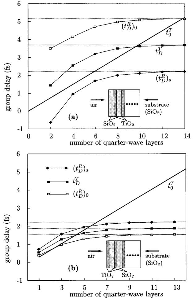
Fig. 3. Group delays as a function of the number of layers for (a)  $(2p)$  and (b)  $(2p + 1)$  quarter-wave layers, assuming normal incidence,  $\lambda_0 = 800$  nm, and  $q = 0$ . Horizontal lines, the asymptotic limits of Eqs. (10)–(15). Transmission is superluminal as soon as  $t_D^T$  is smaller than  $t_0^T$ .
