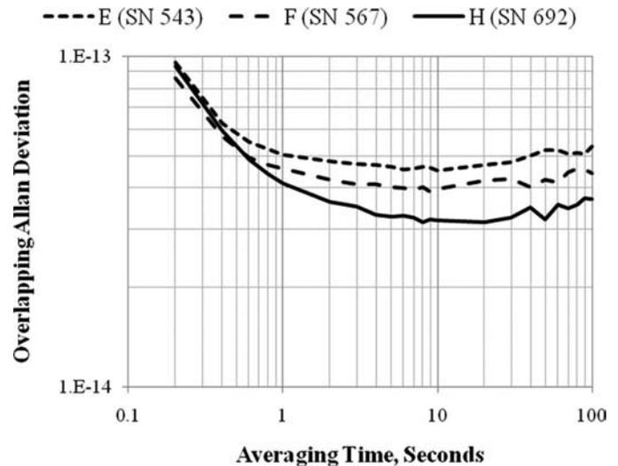
Fig. 5. Frequency stability of the reference oscillators of Oscilloquartz S.A., Neuchâtel, Switzerland.
