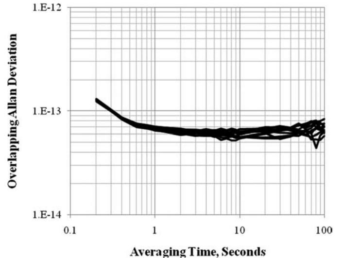
Fig. 2. Frequency stability of the E-F oscillator pair.
