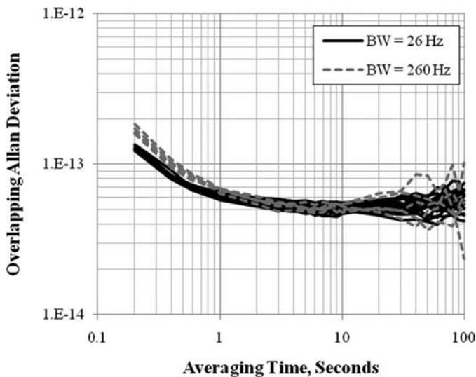
Fig. 4. Frequency stability of the F-H oscillator pair.
