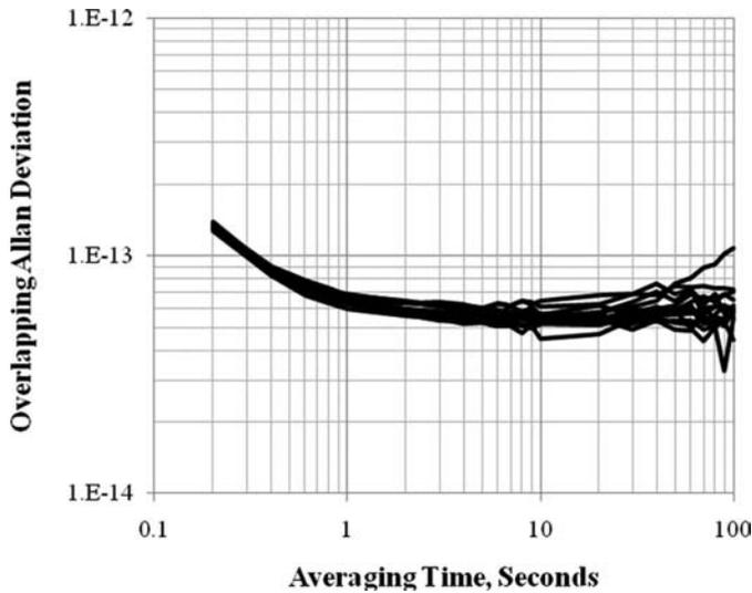
Fig. 3. Frequency stability of the E-H oscillator pair.
