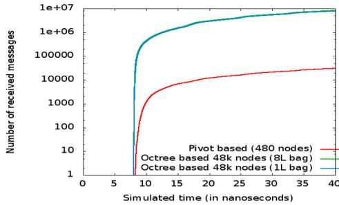
Figure 2: Received messages in function of the simulated time (for 480 nodes pivot based simulation and for 48 000 nodes octree based simulations)
