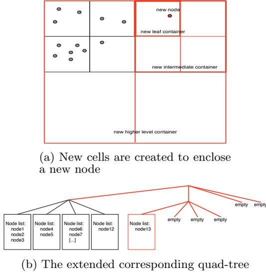
Figure 1: 2D illustration: extending the quad-tree to include a new outside node
